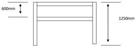
Uprights and rails: upright MUST have a base that is staked into the ground, uprights and rails can be round, rectangular or square.
