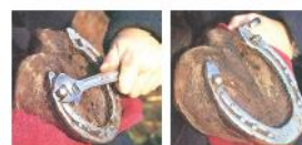
Left: studs must be securely fitted, use the right tools for the job. You can buy studs in a kit with the required tools. Right: The finished job. The inner stud is smooth and rounded for safety while the outer stud is pointed to give more grip.
